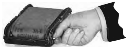
FIG. V. Turning the Key to Bind Paper on Reel.
