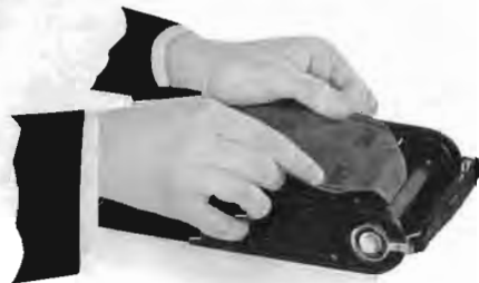
FIG. IV. Threading Red Paper into Reel.
