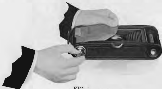
FIG. I. Holding Red Paper Taut while Turning Key.
