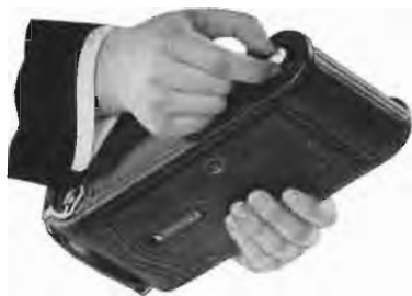
FIG. II. Drawing Out a Spool Pin.
